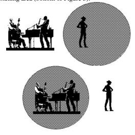
Figure 3 Two equivalent holophonic setups: by surrounding either the listener (top), or the primary sources (bottom).
