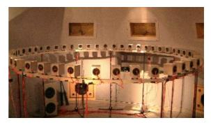
Figure 5 Quasi-circular 48-speaker array for WFS and HOA rendering experiments at the France Telecom R&D Labs
