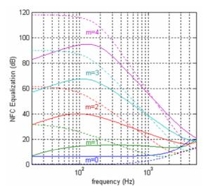
Figure 15 Near Field Compensated Equalization (29) involved in sphere microphone processing  $(R_{\rm mic}=5\text{cm}, R_{\rm spk}=1\text{m})$ . Cont. lines: ideal cardioid sensors; dotted lines: pressure sensors over a rigid sphere.
