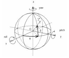
Figure 6 Spherical coordinate system, with the three elementary rotation degrees
