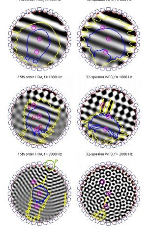
Figure 17 Reconstruction of monochromatic plane waves with HOA and WFS. Blue/dark and yellow/bright contours enclose well-reconstructed areas with error tolerance of resp. 20% and 50%.
