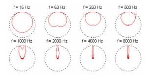
Figure 14 Equivalent pickup directivities or panning laws (normalized absolute values) for  $\rho=\infty$  (plane wave) and  $R_{spk}=1.5m$ , and with "basic" ( $g_m=1$ ), 2D, 15<sup>th</sup> order rendering with Near Field pre-Compensation.
