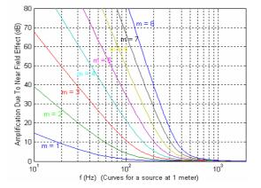
Figure 12 Low frequency infinite boost (m×6 dB/octave) of ambisonic components due to near field effect
