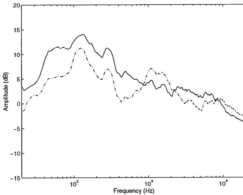
Figure 26: SPL of the right channel measured with (solid line) and without equalizer (dashed line).
