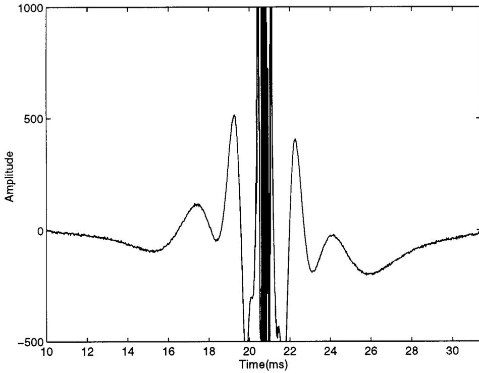
Figure 22: Impulse response of the multi-rate equalizer (detail).
