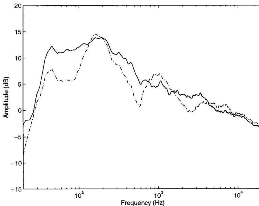
Figure 25: SPL of the left channel measured with (solid line) and without equalizer (dashed line).
