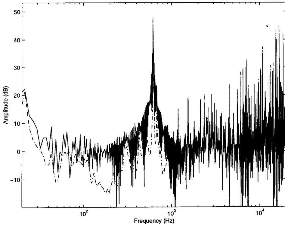
Figure 4: Amplitude of  $H_{inv}(f)$  (dashed), and the filter obtained with 8001 taps (solid).
