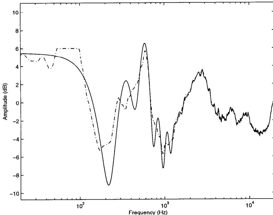
Figure 8: Harmonic response of the designed equalizer (Amplitude).
