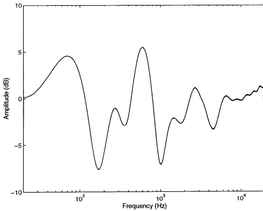
Figure 23: Frequency response of the multi-rate equalizer (Amplitude).
