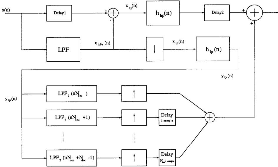
Figure 15: Block diagram of the multi-rate equalizer architecture.
