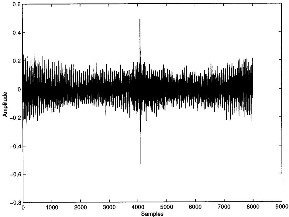
Figure 5: Impulse response of the synthesized filter (8001 taps).
