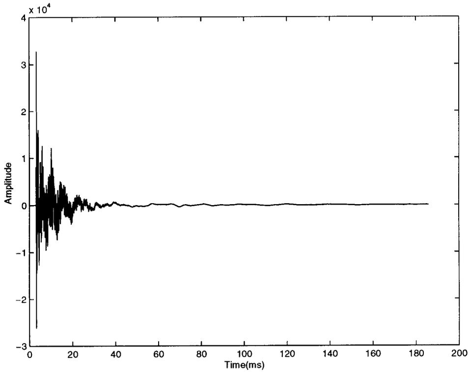
Figure 3: Impulse response of the left channel of a Fiat Lancia Delta (normalized data).
