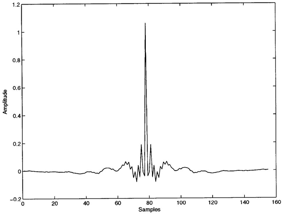
Figure 10: Impulse response of  $h_{ip}(n)$
