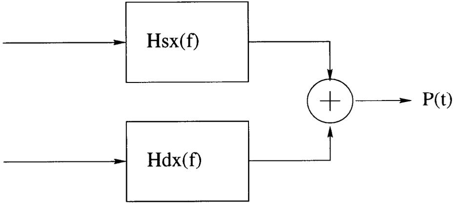
Figure 2: Linear model of the Hi-fi car system.
