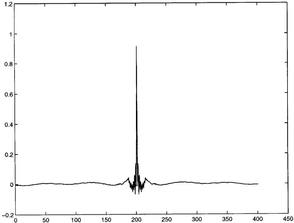
Figure 9: Impulse response of the designed equalizer.
