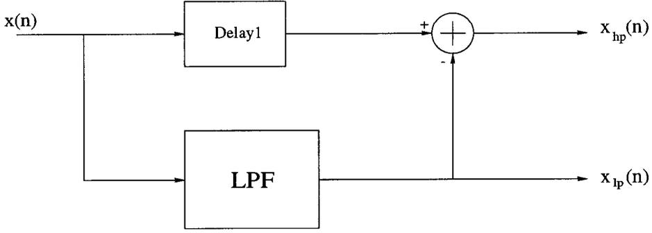
Figure 14: Block diagram of an digital crossover system.
