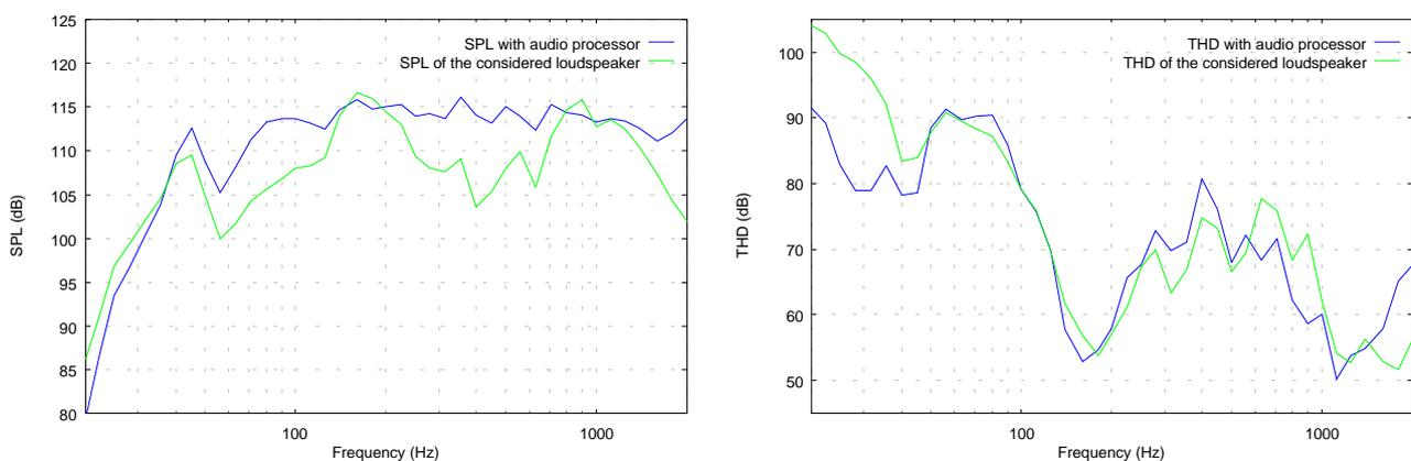
**Figure 2 Comparison between the SPL (a) and the THD (b) of the considered loudspeaker with and without the audio processor.**
