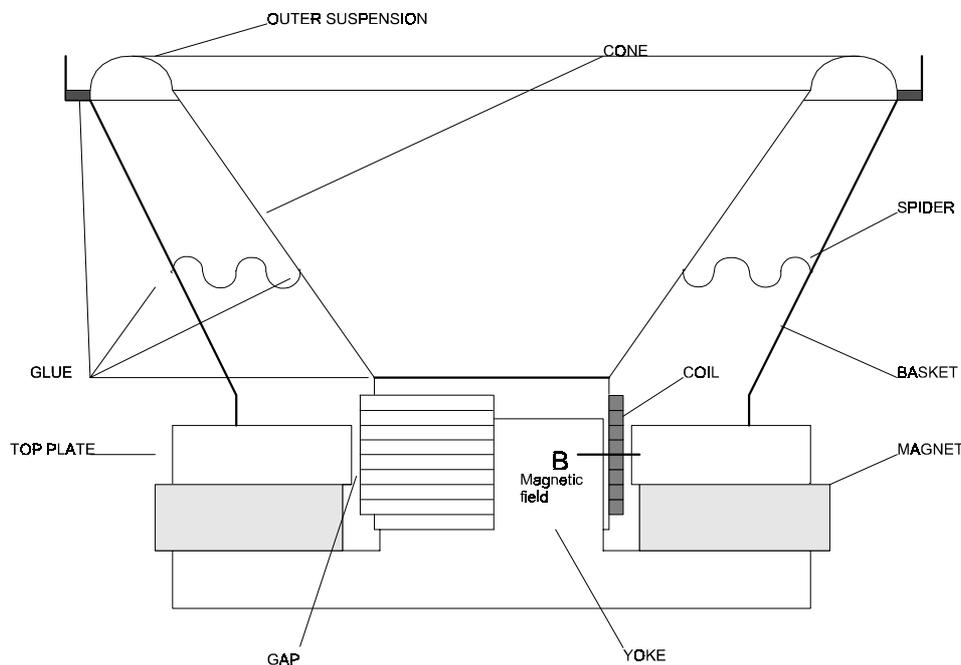
**Figure 1 Basic loudspeaker conformation**
