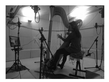
Fig. 2. Positioning of the musicians during the recordings: around the performer the microphone array, on the left the monitor with the conductor video.
