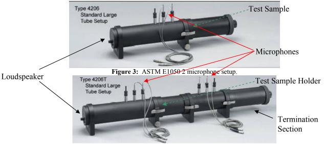
Figure 4: ASTM E2611 4 microphone setup.
