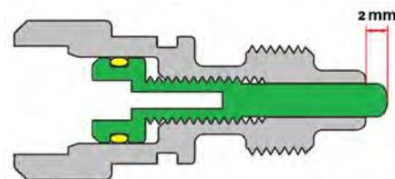
16. Place the o-ring on the adjustment knob and lubricate both o-ring and threads.
