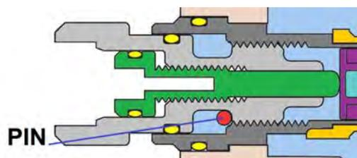
18. Insert the inlet tube assembly inside the case, placing the lever facing the diaphragm. Check if the injection hole is facing the mouthpiece tube.
