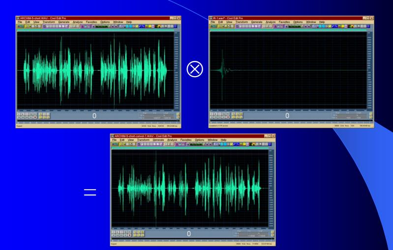
Convolving a suitable sound sample with the linear IR, the frequency response and temporal transient effects of the system can be simulated properly
