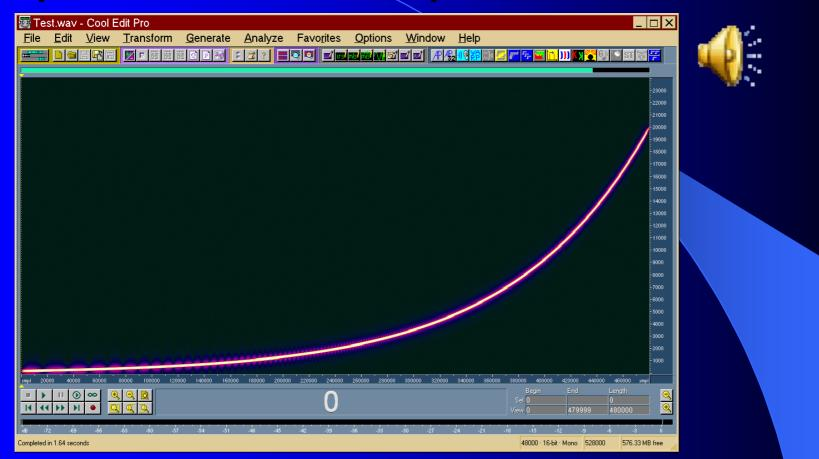
The excitation signal is a sine sweep with constant amplitude and exponentially-increasing frequency
