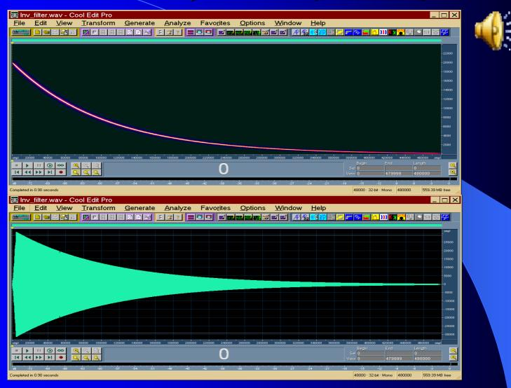
The deconvolution is obtained by convolving the raw response with a suitable inverse filter
