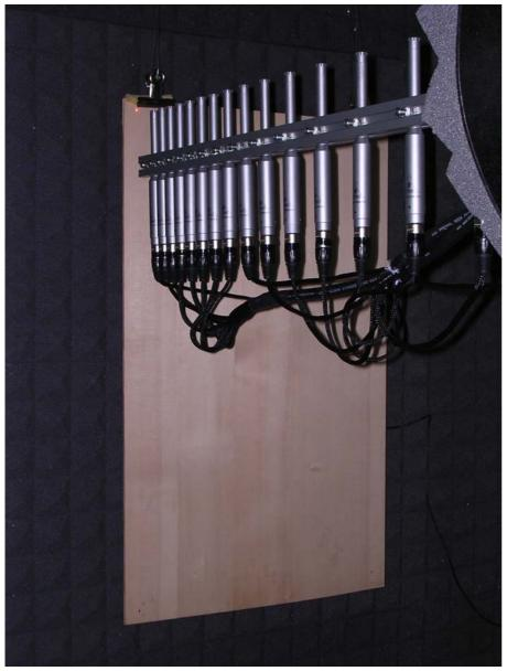
• The wood panel is excited by a small piezoelectric transducer
