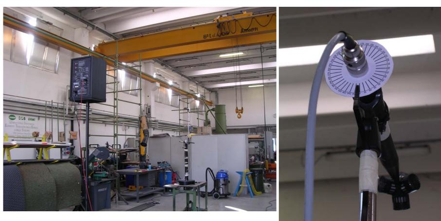
84 IRs were measured, uniformly scattered around a sphere
