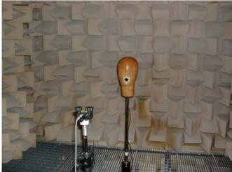
The mouth simulator was built inside a wooden dummy head, employing low-cost parts. Its compliance with the ITU recommendation was confirmed by means of anechoic directivity tests.
