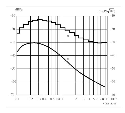
The spectrum of the emitted test signal should correspond to the prescriptions of ITU T-P50
