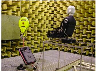
A B&K type 4100 head and torso simulator was selected, after careful comparative tests performed in an anechoic chamber, which demonstrated its superiority to other binaural microphones (Neumann, Cortex, Head Acoustics) when employed for measuring impulse responses
