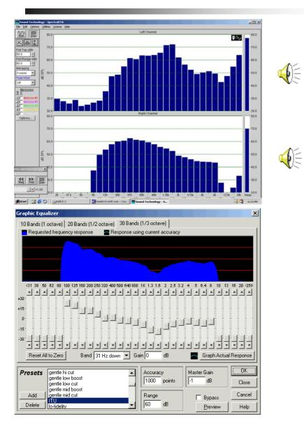
The MLS signal is prefiltered, so that the frequency response, measured at 1m in front of the mouth, complies with the IEC spectrum.
