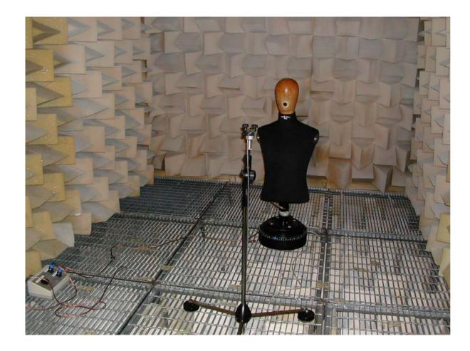
The mouth simulator was built inside a ellipsoidal dummy head, employing lowcost parts. Its compliance with the ITU recommendation was confirmed by means of anechoic directivity tests.
