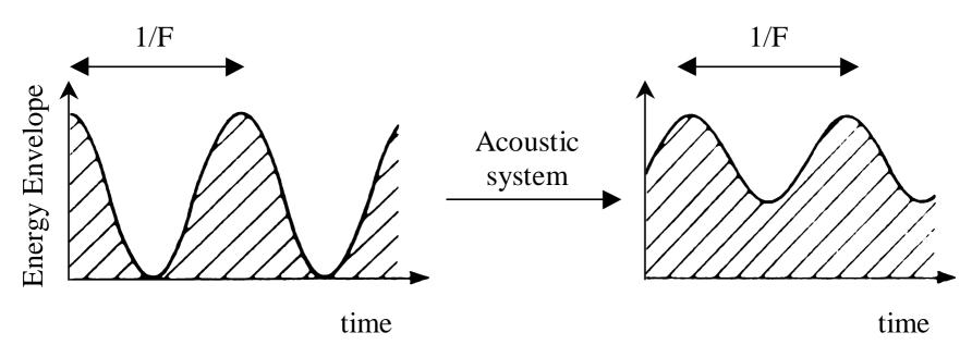
The STI method is based on the MTF concept: a carrier signal (one-octave-band-filtered noise) is amplitude modulated at a given modulation frequency with 100% modulation depth. At the receiver, the modulation depth is reduced, due to noise, reverb, echoes, etc.
