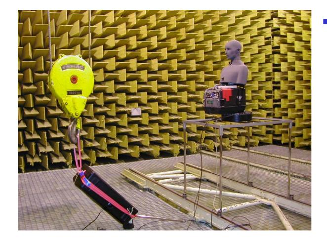
A Cortex head and torso simulator was selected, after careful comparative tests performed in an anechoic chamber, which demonstrated its superiority to other binaural microphones (Neumann, B&K, Head Acoustics)
