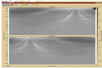
The simmetry revealed to be quite good, and the listening test of the sequence of impulse responses gives the impression of a pulsive source rotating around.
