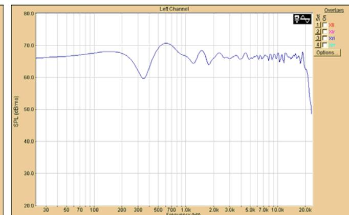
Measured transfer function of Front-Left loudspeaker
