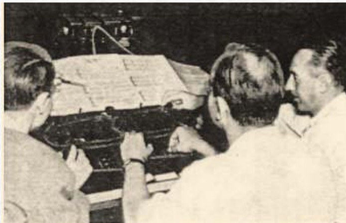
FIG. 13. View of the 3-channel mixing position used in scoring the Fantasia vocal numbers at Burbank. (Messrs. Hawkins, Hissrich, and Marr.)
