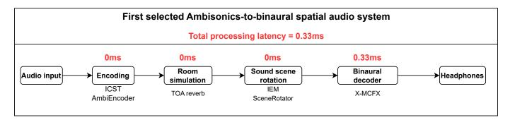
Fig. 3. Representation of the first spatial audio system we selected among the different SAPs, which allows having a SAPs system with the first lowest processing latency to make the Ambisonics-to-binaural workflow. *Audio Input* means the digital audio's real-time input signal (e.g., guitar, bass, vocals).
