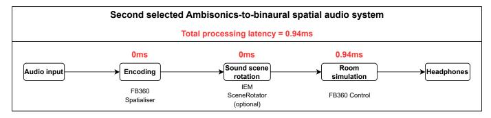
Fig. 4. Representation of the second spatial audio system we selected with the SAPs taken mainly from the FB360 suite, which allows having a SAPs system with the second lowest processing latency to make the Ambisonics-to-binaural workflow. *Audio Input* means the digital audio's real-time input signal (e.g., guitar, bass, vocals).
