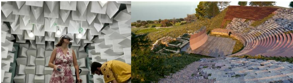
Figure 4 – a) Set-up for listening test in the anechoic room at Politecnico di Torino.
