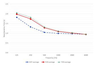
Fig. 6. Measured reverberation time.
