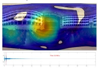
Fig. 11. Acoustical map showing early reflections of the sound energy.
