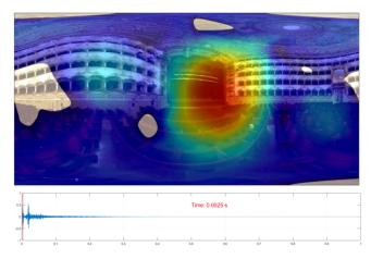
Fig. 10. Acoustical map showing the direct sound arriving at the receiver.
