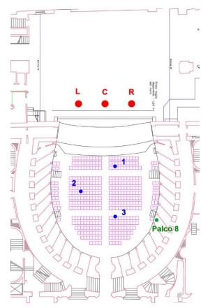
Fig. 4. Source and receiver positions during the acoustic measurements.
