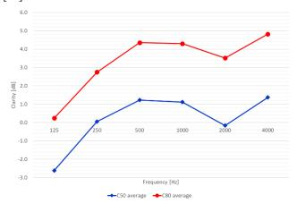
Fig. 8. Measured results of clarity indexes ( $C_{50}$  and  $C_{80}$ ).
