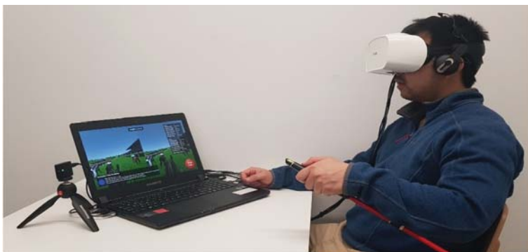
FIGURE 3. AUDIO-VIDEO RENDERING over a head-mounted display. The portable system offers a fully immersive experience for historic reconstructions using either real-time, game-like explorations, or high-quality 360-degree video playback. (Adapted from B. Horan et al., BMC Psychol. 8 , 61, 2020.)
