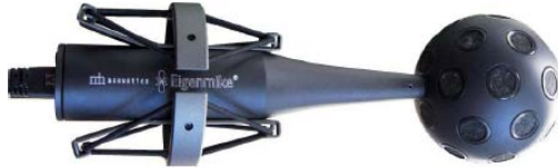
Figure 1: The 32 capsules spherical array (Eigenmike).
