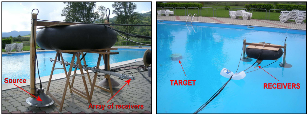
Fig. 6: Active sonar - source and array of receivers set-up(left) and test in the pool (right).
