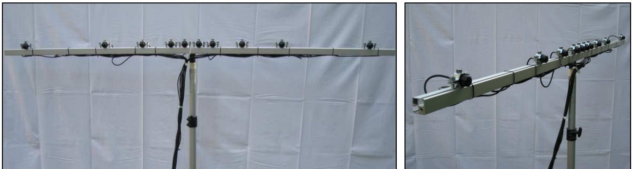
Fig. 1: Ten-hydrophone arranged in the Non-Uniform Linear Array.
