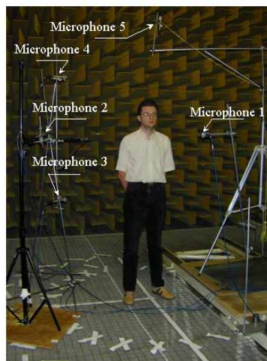
Figure 4 : Illustration of the set-up for the directivity measurement.
