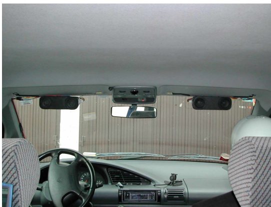
Figure 3: Position of loudspeakers in stereodipole configuration.
