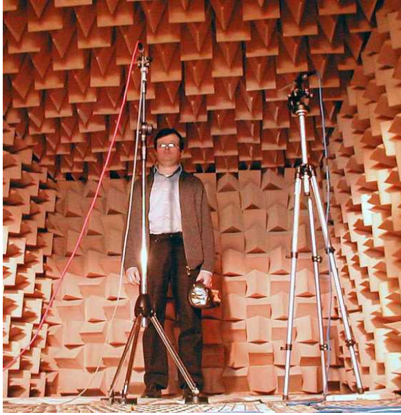
Fig. 4 – real speaker in anechoic room with two microphones for determining his voice's directivity
