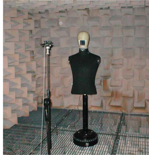
Fig. 2 – Parma University's artificial mouth inside the anechoic chamber on a computer-controlled rotating table
