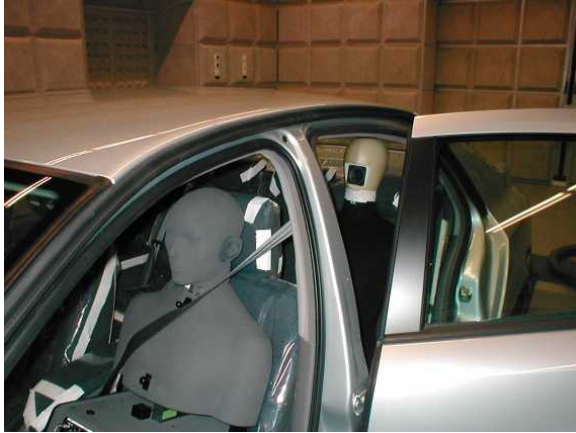
Fig. 1 – measure of STI inside a car using artificial mouth in the back seat and artificial listener in driving position
