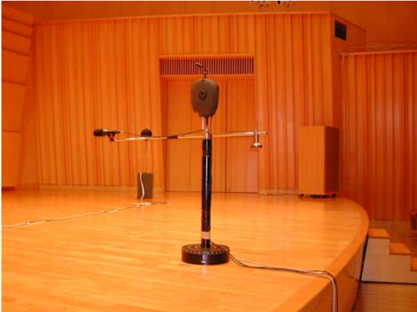
Figure 6: The microphones over the rotating table.
