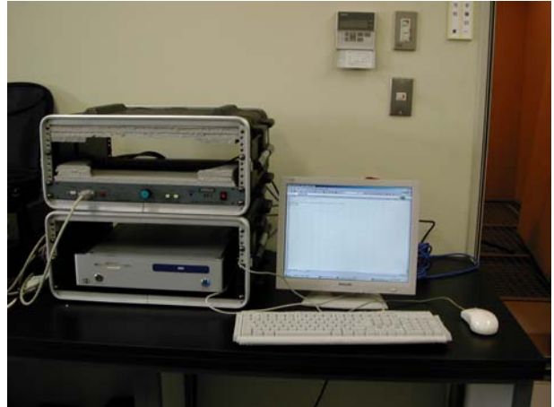
Figure 8: Liquid-cooled PC (FutureClient).
