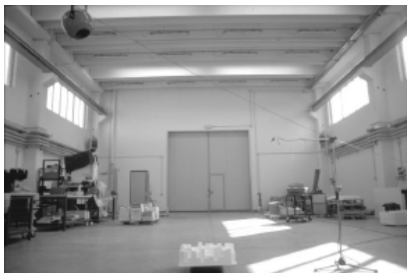
FIGURE 2. Setup of the acoustical apparatus for the measurements with the Vorlander-mommertz free field method
