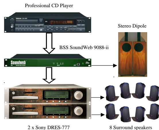
Fig. 29 – Hardware Ambiphonics system
