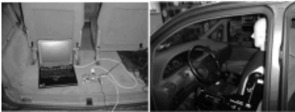
Figure 17 Citroen Evasion cockpit. Dummy head in the driving position (right) and Digital audio processor (left).
