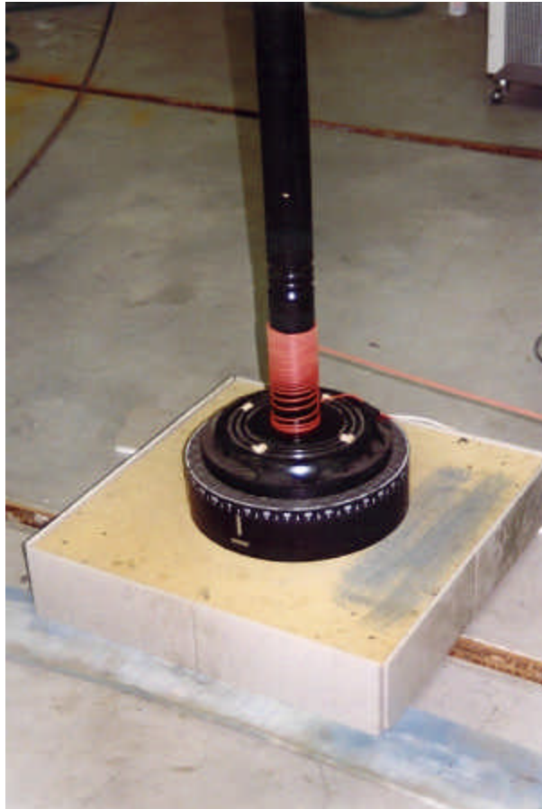
Fig. 7 –Particular of the rotating board with the cable folding around the drum.
