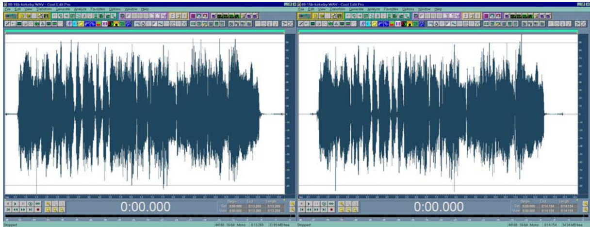
Fig. 6 - Recorded signal and virtual reconstruction obtained by convolution
