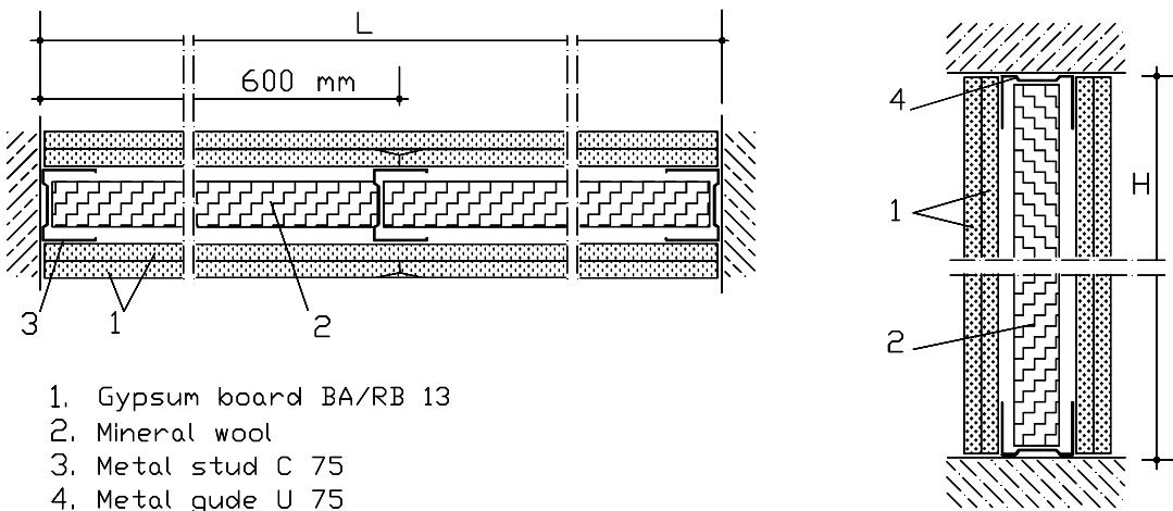
Figure 2: Horizontal and vertical sections of test specimen 2.
