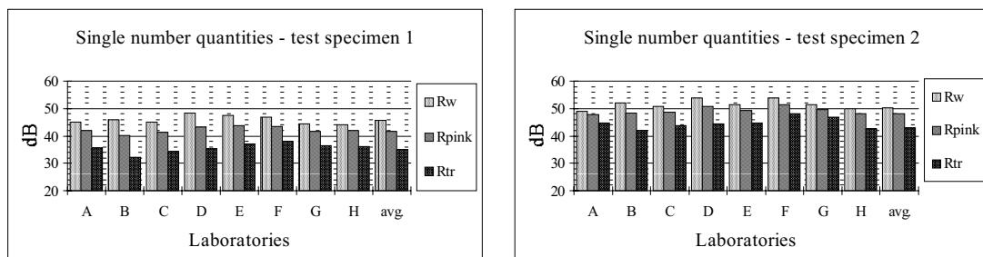
Figure 4: Single-numbers quantities of sound reduction index of specimens 1 and 2:  $R_w$ ,  $R_{pink}$ ,  $R_{traffic}$ .
