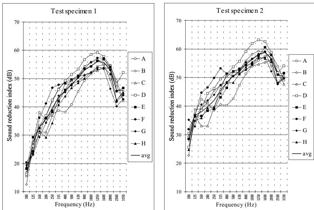
Figure 3: Sound reduction index of specimen 1 and 2 obtained from all the measurements.
