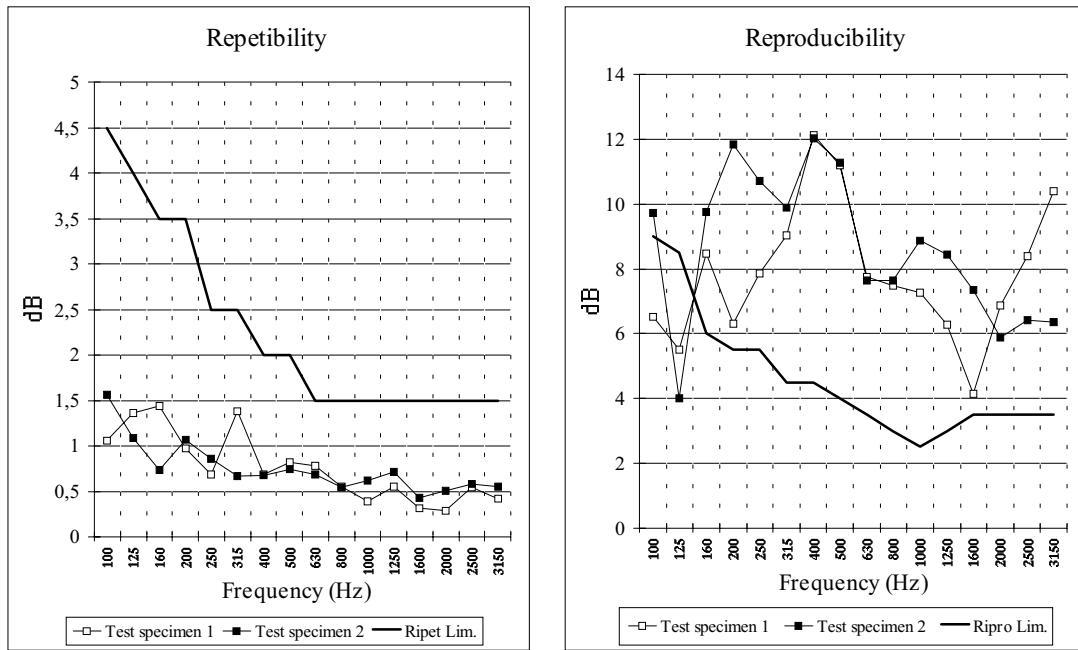
Figure 5: Repeatability "r" and reproducibility "R" values obtained from this interlaboratory test: comparison with the tentative values given in ISO 140-2.
