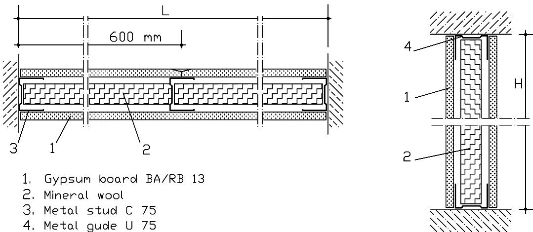
Figure 1: Horizontal and vertical sections of test specimen 1.
