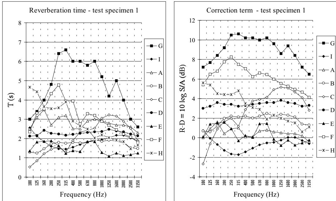
Figure 6: Reverberation time values measured in each of the laboratories and correction term calculated to determine the sound reduction index.
