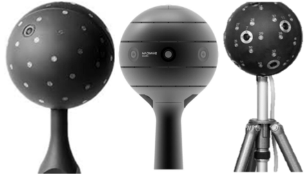
Fig. 1. Three microphone arrays: VisiSonics (left), Sonicam (center) and Bruel&Kjaer (right)
