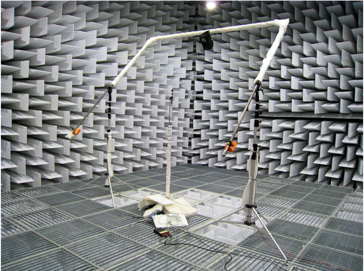
The Brahma probe in the anechoic room of Ferrara University, on the turntable
