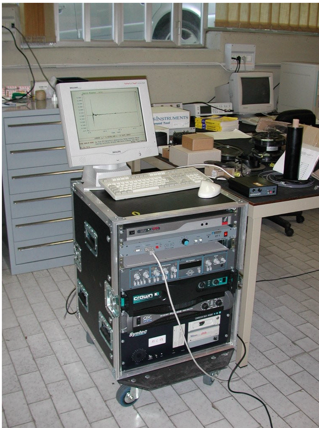
Fig. 3 – the instrumentation rack, containing (from top to bottom): Echo Layla sound board Outline ST-1 control unit Soundfield MK-V preamplifier (not used here) Crown K1 amplifier QSC PLX-1200 amplifier (not used here) Syntec computer (Pentium-II 400 MHz)
