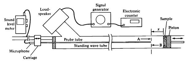
Figure 6. Impedance tube for measuring normal incidence absorption coefficient
