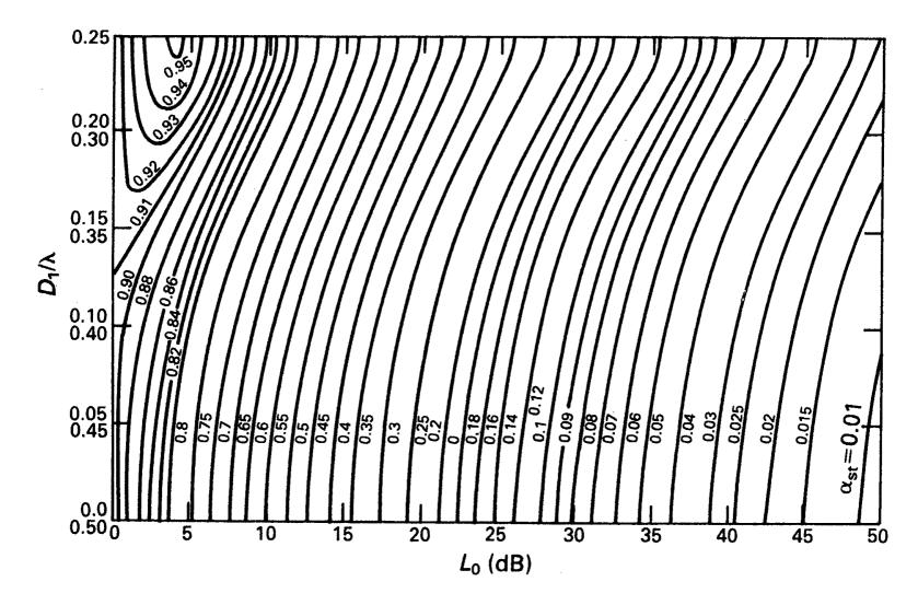
**Figure A4.2** A chart for determining the statistical absorption coefficient  $\alpha_{\text{stat}}$  from measurements in an impedance tube of the standing wave ratio,  $L_0$ , and position  $D_1/\lambda$  of the first minimum sound pressure level.  $\alpha_{\text{stat}}$  is shown parametrically in the chart.
