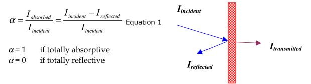
Figure 2. Sound striking an absorbing wall
