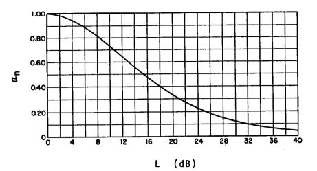
Figure 6.2 Chart showing the relation of the normal incidence absorption coefficient  $a_n$  to the difference in decibels L between the measured maximum and minimum sound levels.
