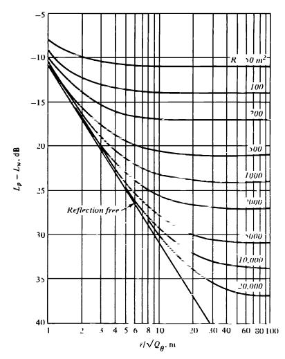
Figure 12. Difference between the sound pressure level and the sound power level in a room as a function of the room constant  $R_T$ , the distance from the source r and the directivity factor  $Q_{\theta}$
