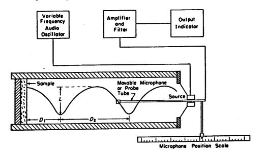
Figure 6.1 Acoustic impedance tube apparatus. (Reprinted with permission from the Annual Book of ASTM Standards, Copyright American Society of Testing and Materials, Philadelphia.
