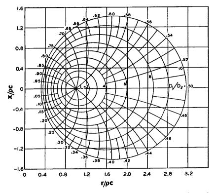
Figure 6.3 Relationship of specific acoustic impedance ratios and measured parameters L and  $D_1/D_2$ , L = 0 to 10. (Reprinted with permissio from the Annual Book of ASTM Standards, copyright American Society of Testing and Materials, Philadelphia.)
