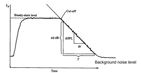
The time required for the sound level to decay 60 dB is called the **reverberation**
