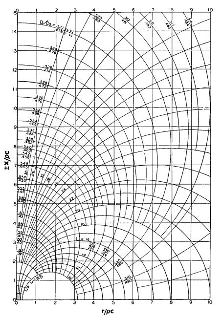
Figure 6.4 Relationship of specific acoustic impedance ratios and measured parameters L and  $D_1/D_2$ , L = 10 to 40. (Reprinted with permission from the Annual Book of ASTM Standards, copyright American Society of Testing and Materials, Philadelphia.)
