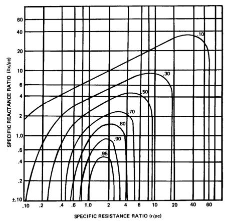
Figure 6.5 The statistical absorption coefficient in terms of the specific acoustic resistance and reactance ratios. (From Ref. 7.)
