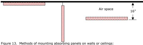
a) hard mounted b) hanging baffle c) air space behind panel
