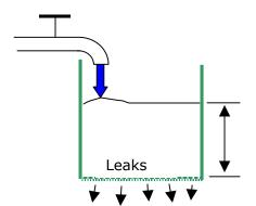
Mean water level (sound pressure in reverb field) = f (input flow rate [sound power] and amount of leaks [absorption] )
