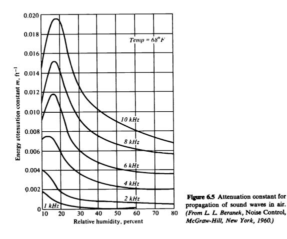
Figure 11. Attenuation for propagation of sound in air
