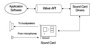
Figure 8. Sound system architecture
