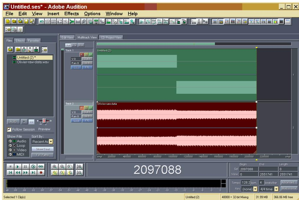
At this point, the Deconvolve Multiple MLS Sequence module is invoked, specifying the proper generation parameters (32 repetitions of the MLS 15B sequence), and that these are 2 measurements (first the left loudspeaker, second the right loudspeaker):
