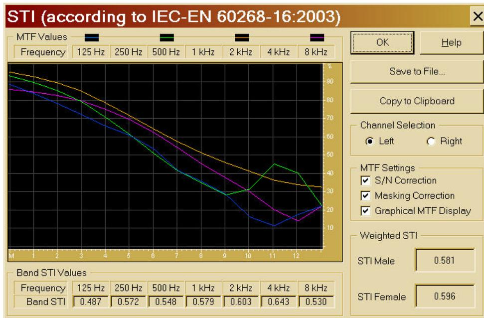
The graphical display of 4 of the 7 octave-band MTF values can be disabled, revealing the complete table of MTF values:
