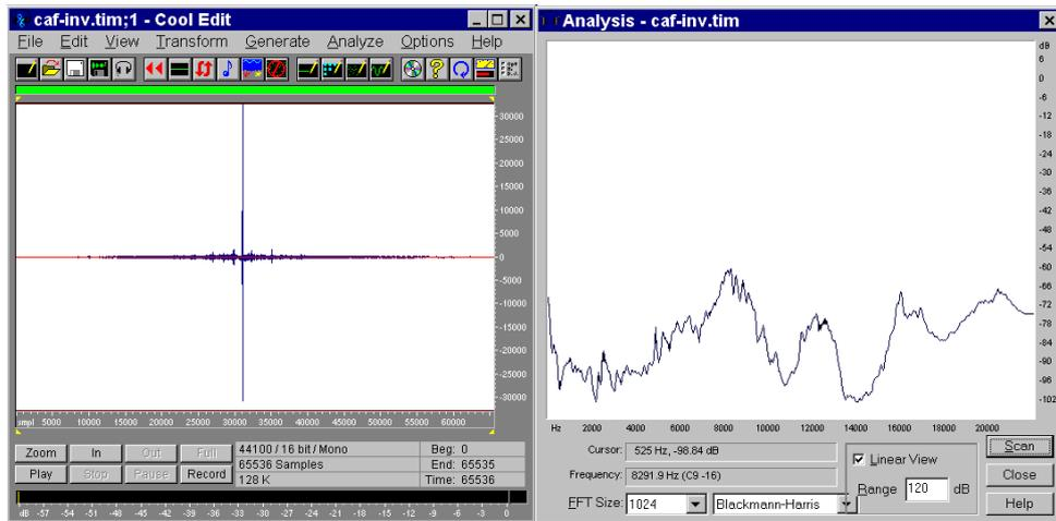
The verification of the proper working of the filter can be done by convolving the original impulse response with it. This is shown in the following pictures: an almost perfect Dirac's delta function has been obtained in the time domain, and in the frequency domain the response is flat.
