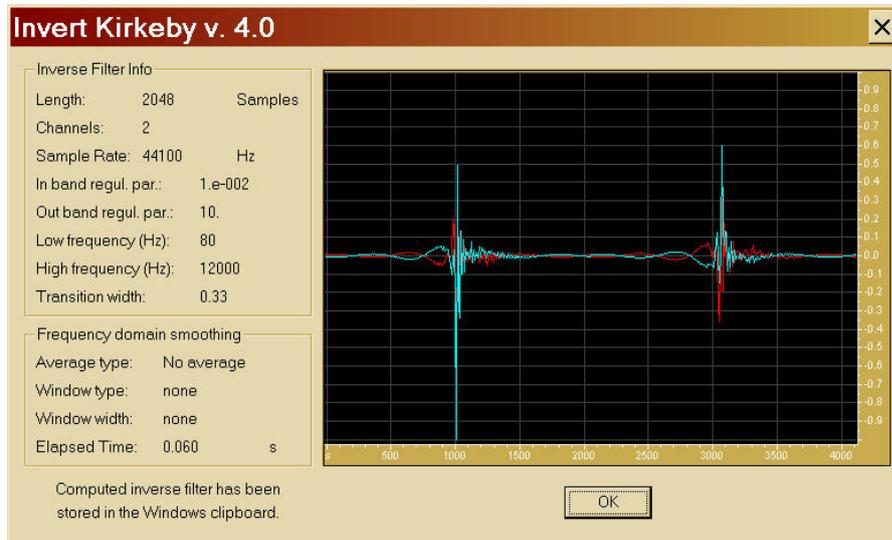
The inverse filters are now in the Windows clipboard, from where they can be pasted to a new waveform:
