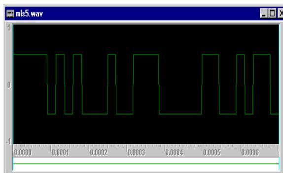
The most versatile of these three generation modules is the Generate Multi MLS. This module was optimized for performing measurements of multi-channel systems (typically 2x2 systems, in which two loudspeaker and 2 microphones are involved, such as the case of a binaural microphone placed in front of a loudspeaker pair). When generating a stereo signal, this module creates first a series of MLS sequence on the left channel, followed by the same signal repeated later on the right channel:
