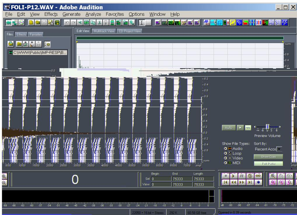
Now we copy this binaural stereo IR to the Windows Clipboard (Edit – Copy). Then we can load an anechoic signal:
