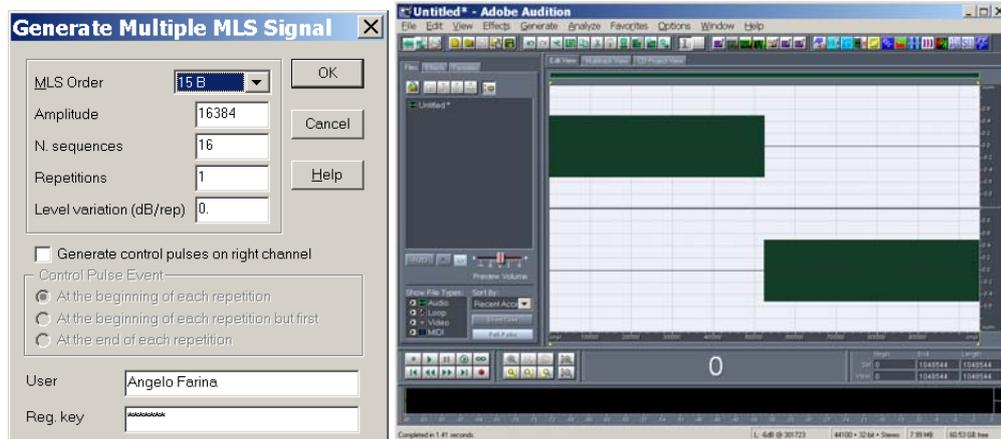
This way, the measurement can be performed playing the stereo signal, and recording the system's response simultaneously; first the left loudspeaker will be excited, followed by the right loudspeaker.
