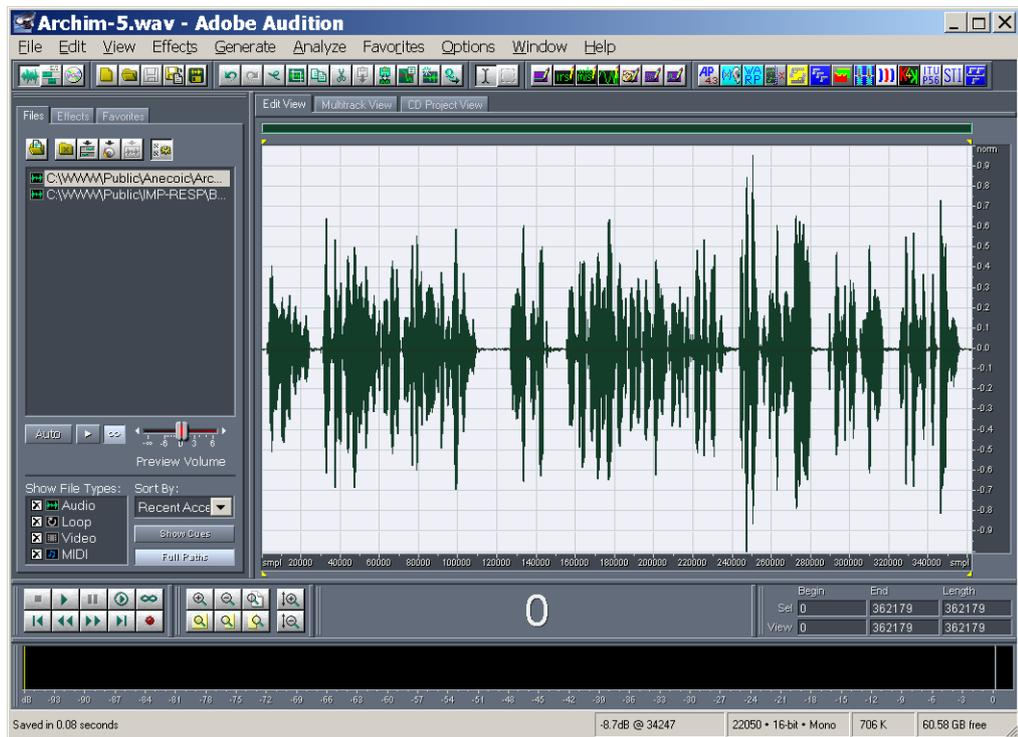
This is a mono file: if we want it to be convolved with the binaural stereo IR, producing a stereo result (auralisation), we need first to convert the waveform to stereo, making use of the standard Audition "Convert Sample Type" function. It is also advisable to extend the bit depth from 16 to 32 bits, because the following convolution will expand significantly the dynamic range:
