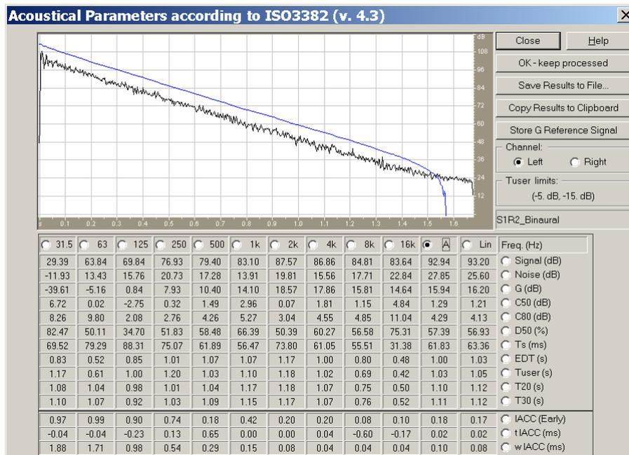
The user can choose to display a plot of the impulse response and of the Schroeder-integrated decay (in blue) at any of the frequency bands, just selecting it. Similarly, the user can switch to the right or left ear display at will.
