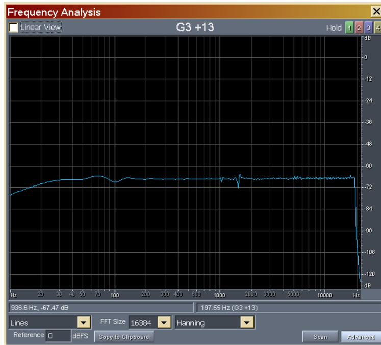
This is only almost flat, due to the limited number of taps employed for the creation of the Inverse Filter. And the frequency smoothing applied to the inverse filter.
