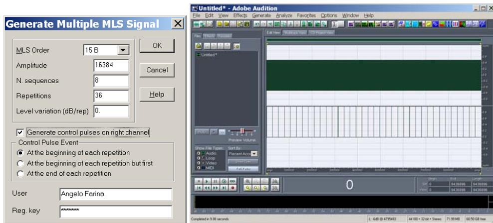
Then the measurement is performed employing the multitrack mode of Audition:
