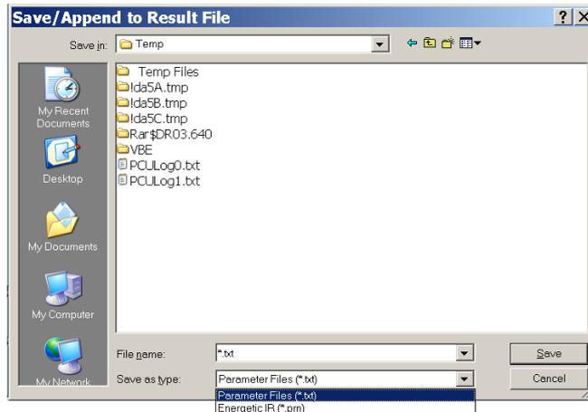
Choosing Parameter Files exactly the same table as stored to the clipboard is saved to a TXT file. Choosing Energetic IR, instead, a PRN file is created, containing a table of energetic values in octave bands, sampled with an 1ms time resolution. Both files can be easily imported in Excel, Matlab or other programs for further processing.
