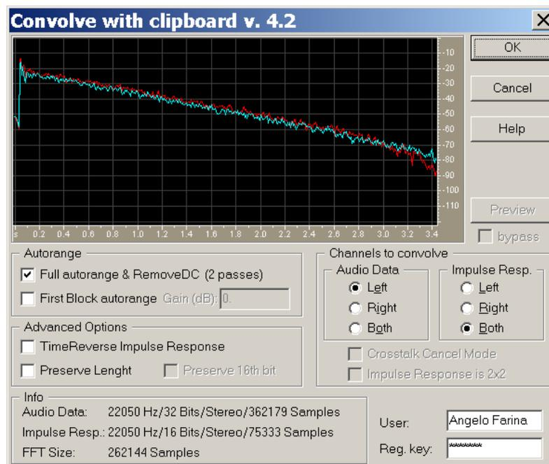
In this case, as it is shown, we want to convolve the Left channel of the current audio data with both the channels of the IR, and we want to perform a full autorange (selecting full autorange makes the "preview" function unavailable). When OK is pressed, the standard Progress Meter of Audition appears, until the convolution process is finished. At this point the final dialog box is displayed, reporting statistics about the convolution process:
