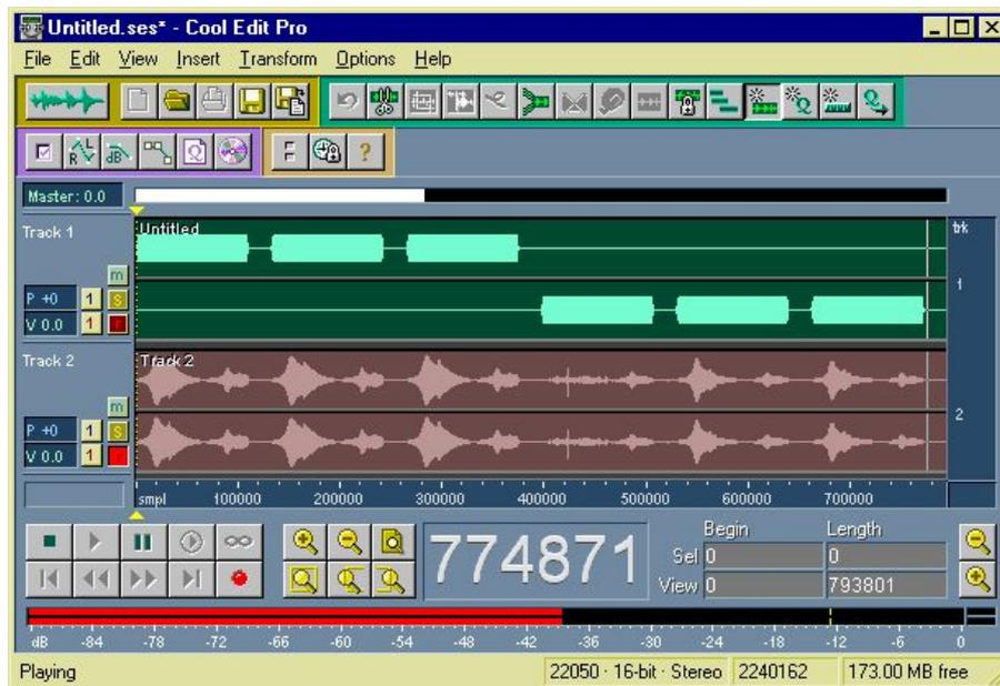
The deconvolution is made, in this case, simply convolving the recorded response (track 2) with the clipboard, where the proper inverse filter was already stored from the **Generate SWEEP Signal** module. This way, the following sequence of raw impulse responses is obtained:
