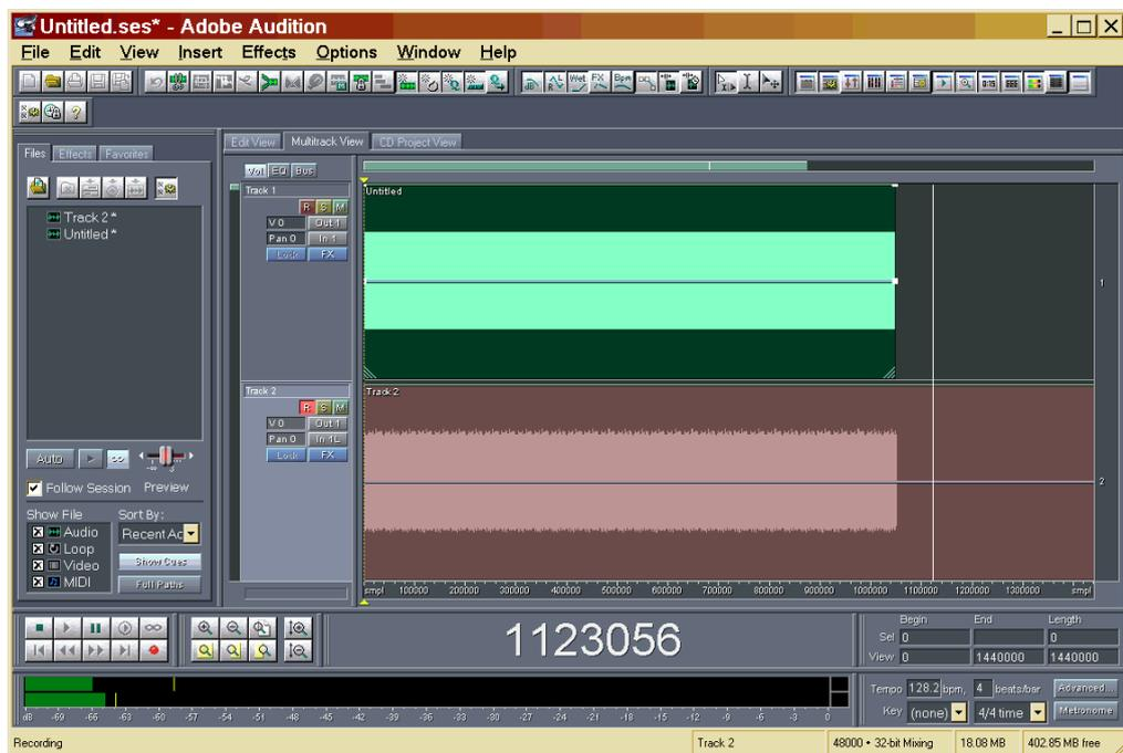
Now Track2 is opened in the Edit View mode (just double-click over it), and the Deconvolve Multiple MLS module is invoked (or the DecoMLS or the DecoRS, if appropriate). The following mask does appear:
