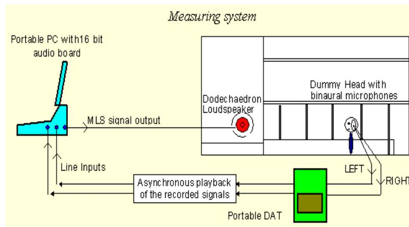
MLS stands for Maximum Length Sequence, IRS stands for Inverse Repeated Sequence. Both these excitation signals are defined as a pseudo-random sequence of binary digits (0 and 1), built with a complex number-theory technique.
