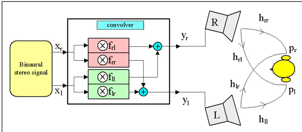
In the general case, the system is not perfectly symmetric, and consequently nothing ensures that the ipsilateral filters  $F_{LL}$  and  $F_{RR}$  are equal, or that the crosstalk filters  $F_{LR}$  and  $F_{RL}$  are equal either.
