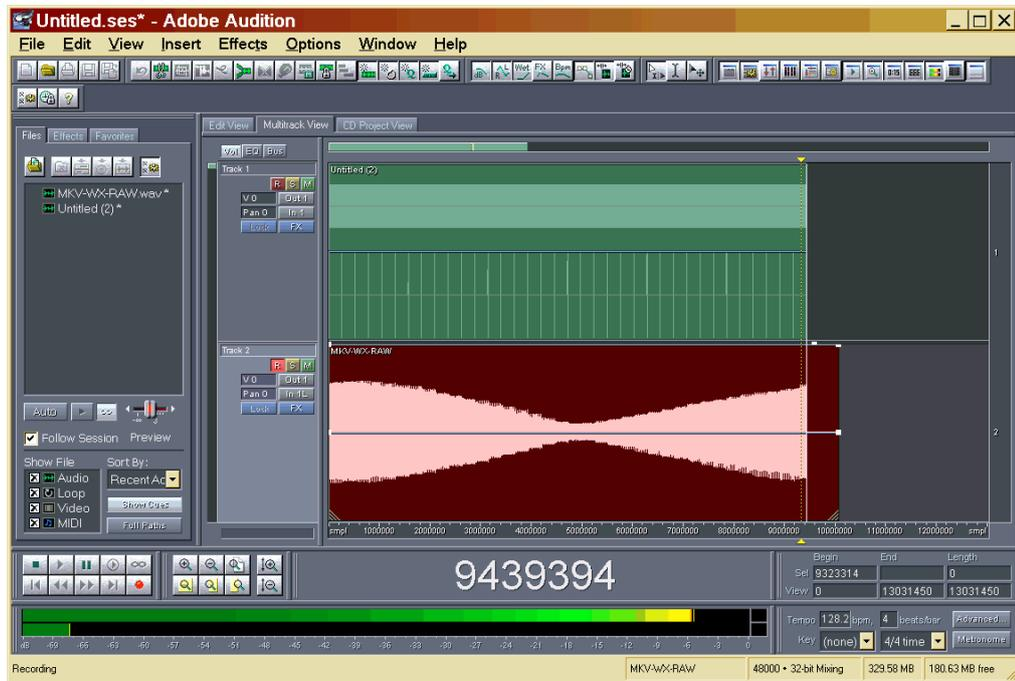
The recorded signal will then be deconvolved employing the Deconvolve Multi MLS Signal module, and the result will be a sequence of 36 impulse responses, one for each angular position.
