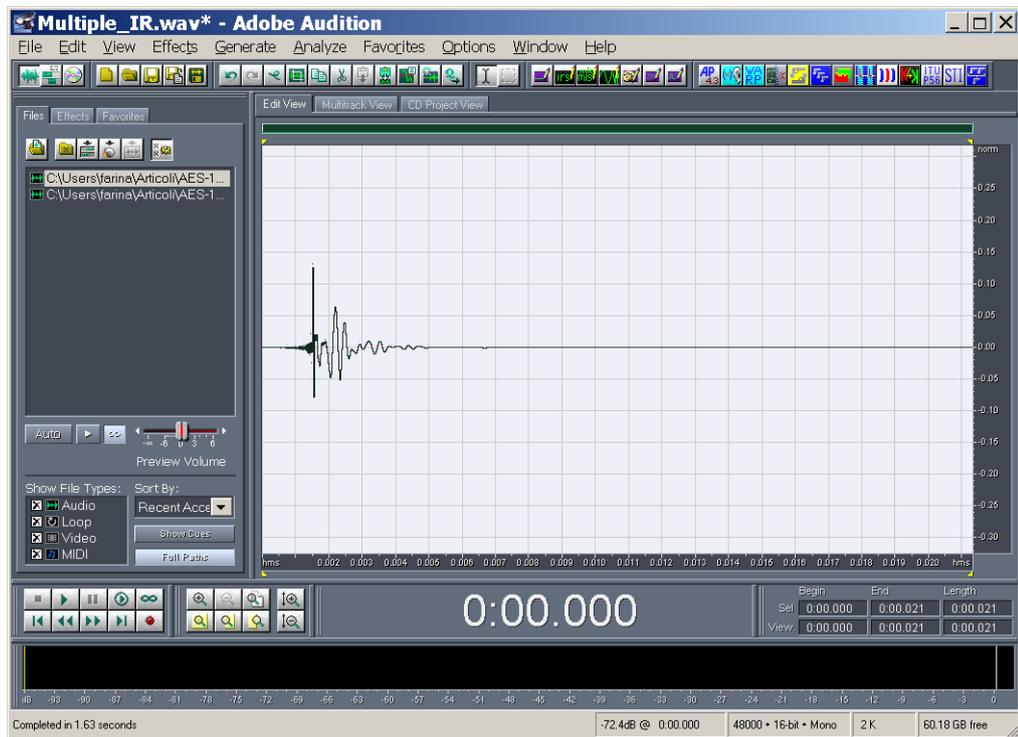
One by one, we can this get a complete extraction of all the harmonic orders, By analyzing separately each of them, the complete harmonic distortion spectrum can be obtained for each order.
