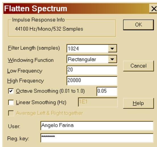
With this dialog box it is possible to select some parameters, which affect the computation of the Inverse Filter.
