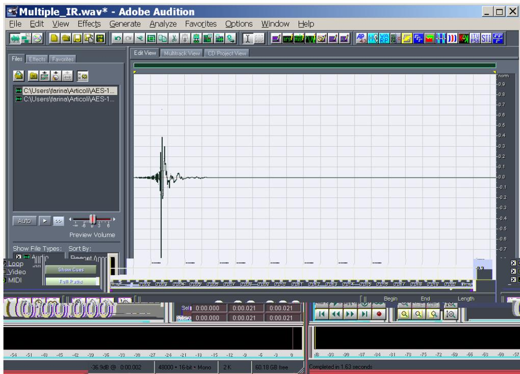
We can now save it, then Undo the IR selection. Starting again from the multiple-IR signal, we can now IR-select, for example, the 3<sup>rd</sup>-order IR:
