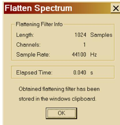
At this point the Inverse Filter has been stored in the Windows Clipboard. Making a Paste-New from the Windows Clipboard, the following signal is recovered:
