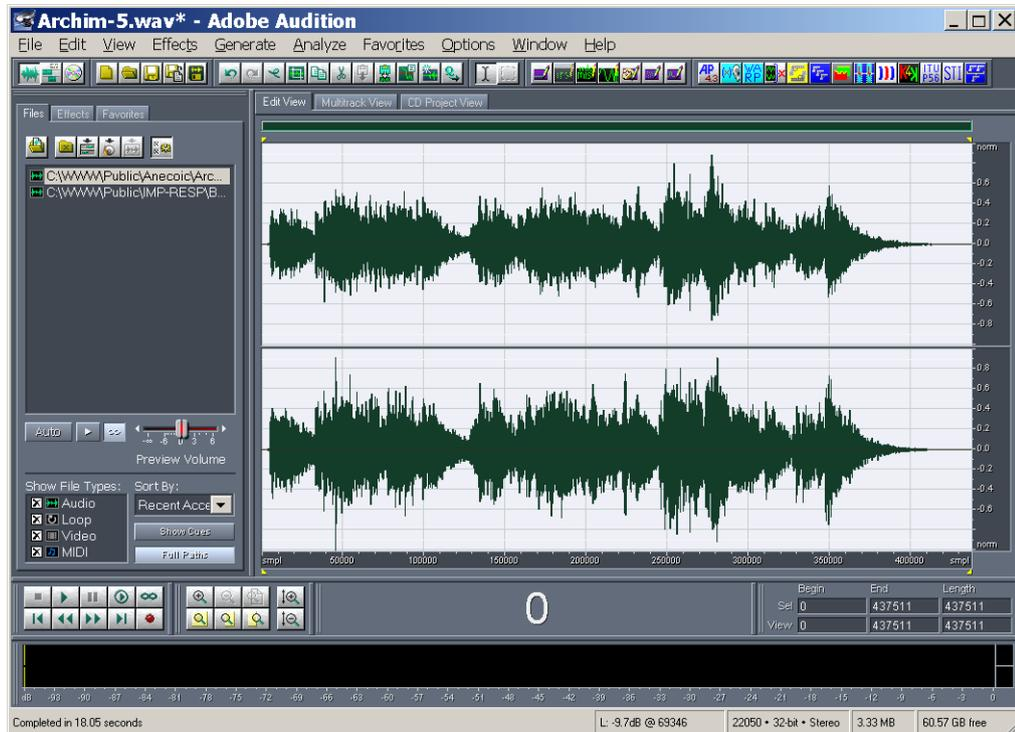
This stereo waveform, obtained by convolution of a mono signal with a binaural IR, is now suitable for headphone listening. If such a binaural signal needs to be reproduced onto a loudspeaker pair, it is necessary to apply a further convolution with a set of properly-designed cross-talk canceling filters. This can be done again with Convolve with Clipboard module.
