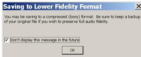
This warning is not true: the TIM format is not lossy, nor compressed: it preserves the complete information contained in the waveform, including true 32-bits (float) depth. The only case in which some data is lost is when the Impulse Response to be saved is longer than 65536 samples, because this is the maximum length allowed by the MLSSA program.
