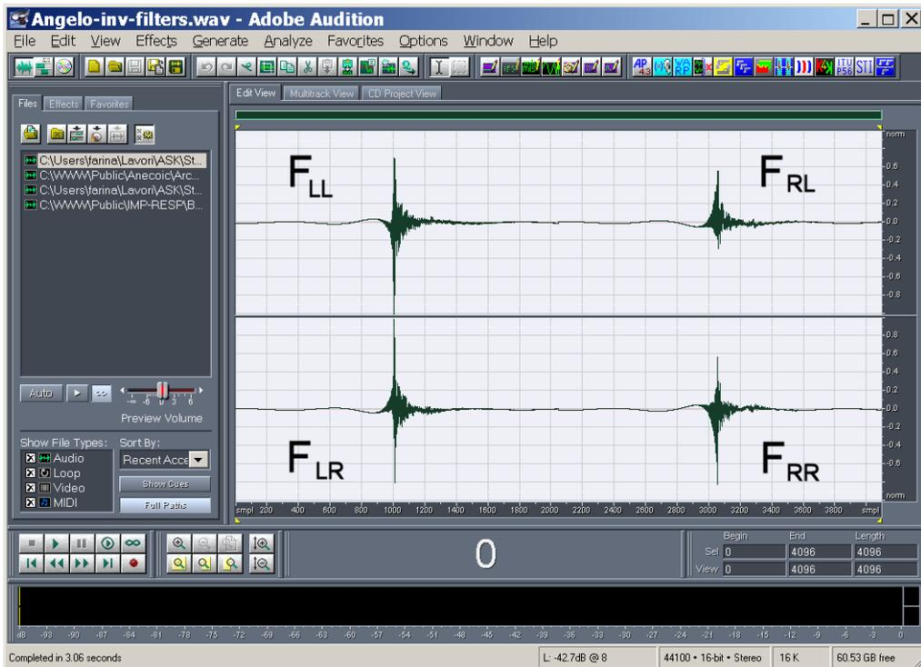
These inverse filters  $F$  need to be loaded into the Windows clipboard before the Convolve with Clipboard module is invoked. Then a binaural recording (or auralization) signal  $X$  is opened, and is convolved with the clipboard, specifying both the Crosstalk Cancel mode Flag and the Impulse Response is 2x2 flag.
