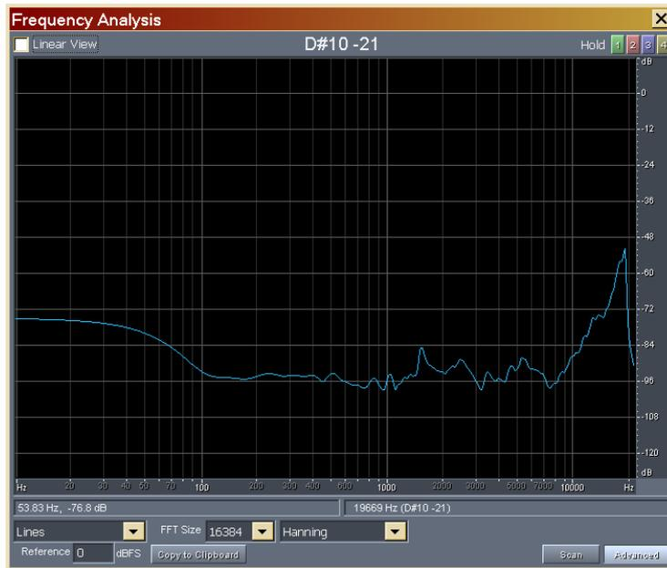
This is roughly the specular image of the original Impulse Response, and thus the recovered signal is the required equalising filter. For verification, if we apply it by convolution to the original signal we obtain the following:
