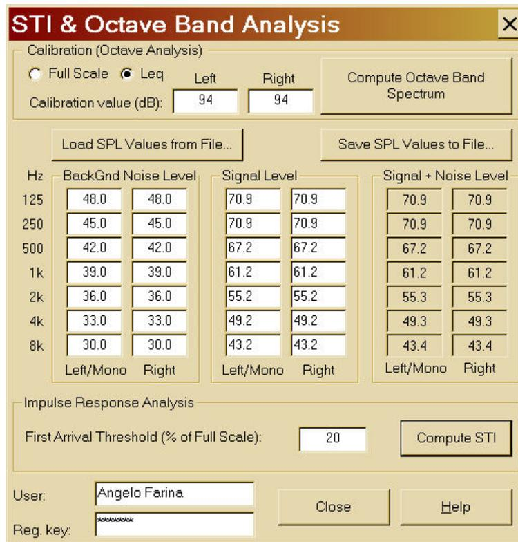
And we specify the Leq value for each of the two channels - then, pressing the button labelled "Compute Octave Band Spectrum", the following result appears:
