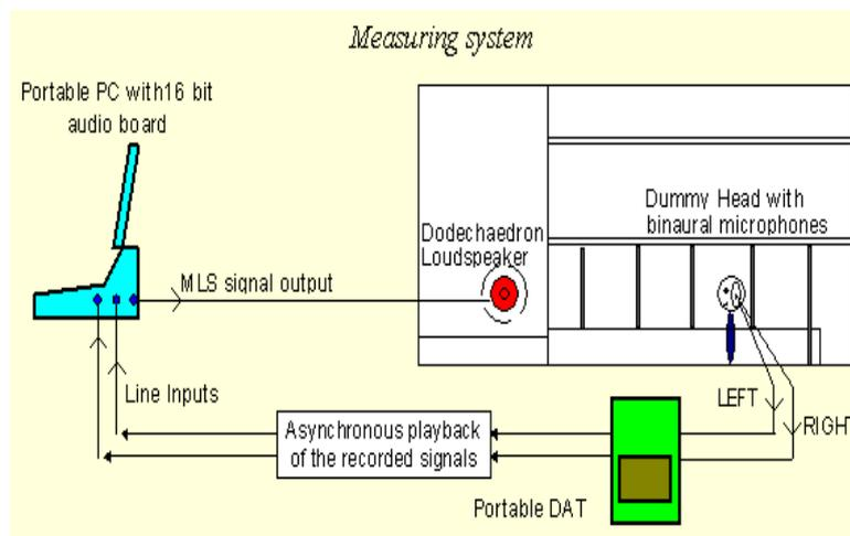
The computer is used for generating the MLS (or IRS) sequence, and for feeding the omnidirectional loudspeaker (or the sound reinforcement system, if this must be included in the measurement). The recording of the response is not made simultaneously to the playback of the signal, for three reasons:
