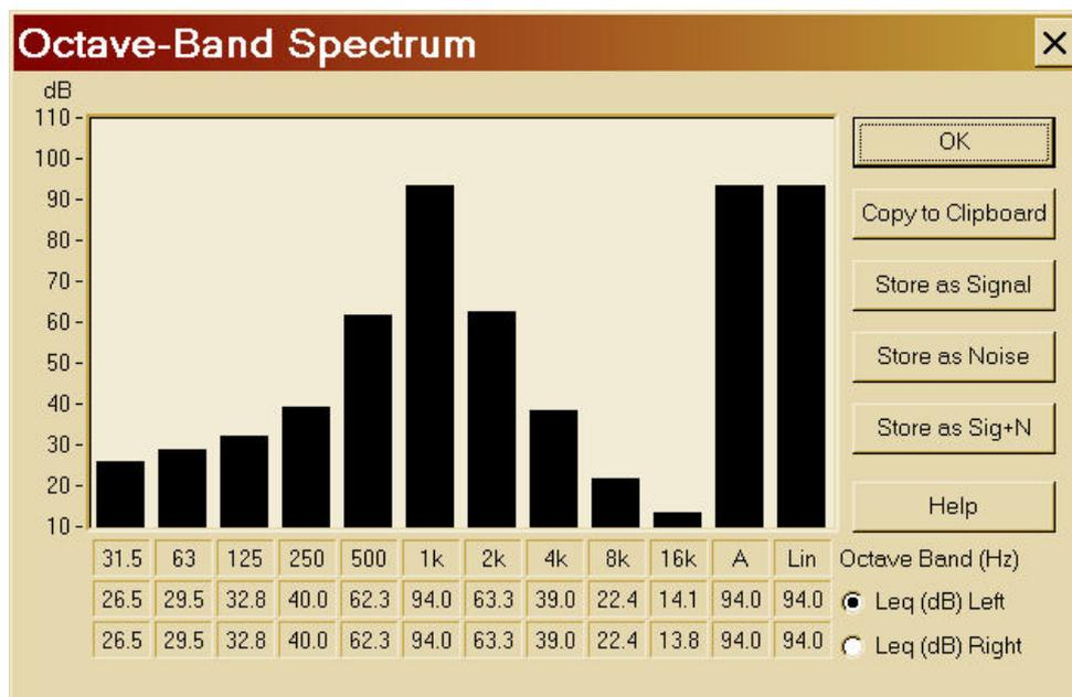
We can press OK. Now the amplitude scale of the STI module is correctly calibrated, and the next time we will not need anymore to specify the Leq value.
