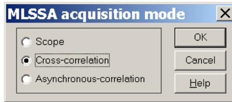
This makes it possible to select the MLSSA acquisition mode which is flagged inside the .TIM file: this way the user can "fool" MLSSA, changing the acquisition mode after a measurement is made, thus making it possible to perform computations that MLSSA does not allow for certain kinds of data (for example computing the Acoustical Parameters from Scope data).
