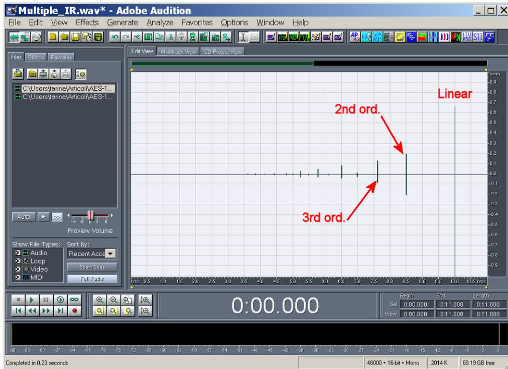
The last peak is the linear impulse response, the preceding ones are the harmonic distortion IRs of increasing orders...
