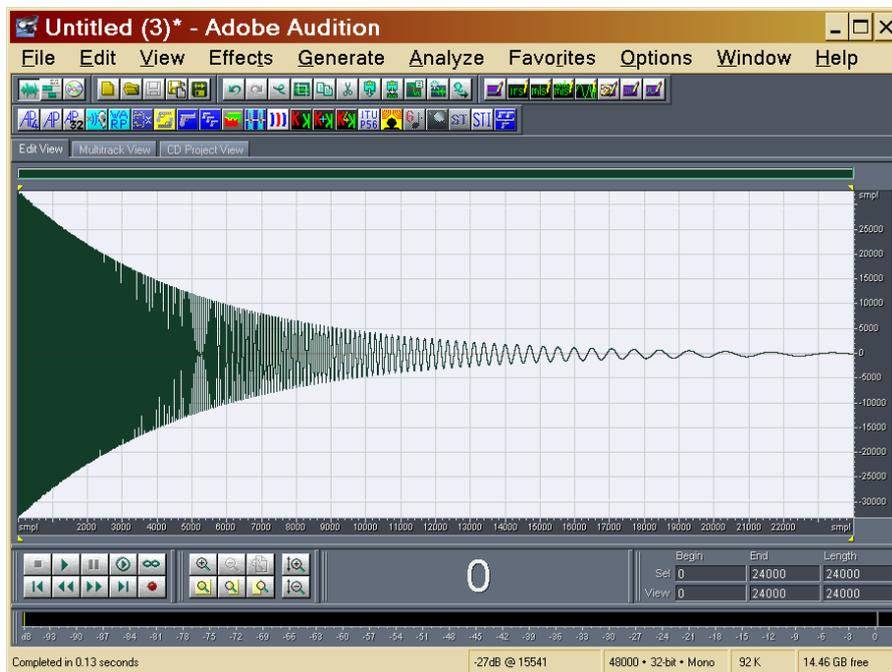
For recovering the impulse response, the recording made after the excitation of the system with the sweep signal must simply be convolved with the inverse filter. This is
